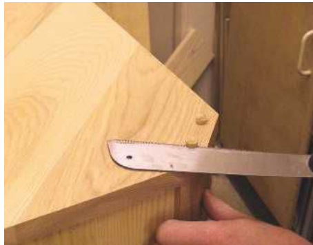
▲ Pic.16 Glue the dowels and hammer them in. Then cut them nearly flush and plane them smooth
